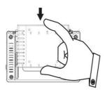
To remove the battery pack from the DVT, locate the locking tab at the top of the pack and press in. Push the pack upwards until tabs are clear of the DVT.
